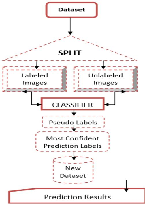
**Figure 2:** Semi-supervised Framework for safe landing of UAVs.
