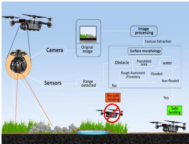
**Figure 1:** Autonomous Safe Landing Detection System
